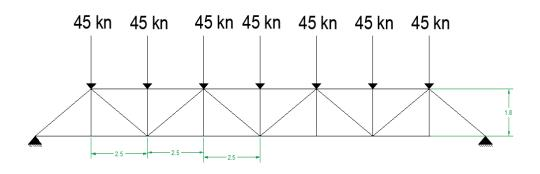
truss from 8 spans each span 2.5 m length, height of truss is 1.8 m ,load
